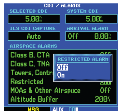
Figure 10-31 Restricted Alarm Window
