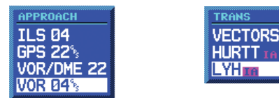
Figure 6-11 Approach and Transitions Windows
